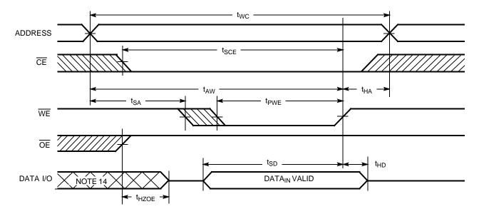
**Notes:** 12. Data I/O is high impedance if  $\overline{OE} = V_{IH}$ . 13. If CE goes HIGH simultaneously with WE going HIGH, the output remains in a high-impedance state. 14. During this period the I/Os are in the output state and input signals should not be applied.
